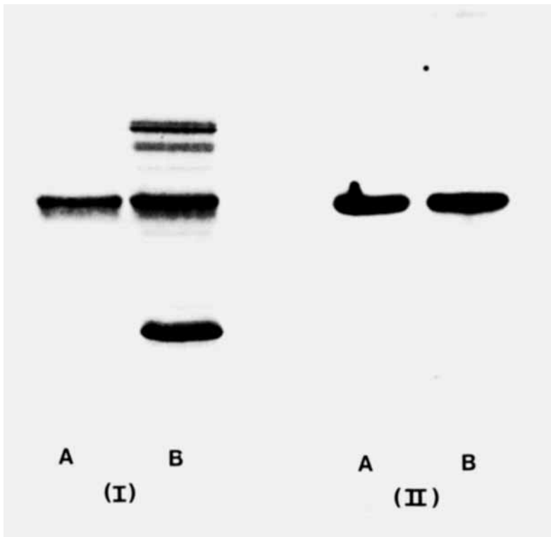
Fig. 3. Active site labeling of esterase with diisopropyl phosphofluoridate. Samples of purified esterase (A) and crude tissue extract (B) were incubated with [ ^3\text{H} ]DFP and subsequently electrophoresed on 15% polyacrylamide gels containing 1% SDS. I) Coomassie blue staining pattern; II) autoradiogram of the [ ^3\text{H} ]labeled proteins.
